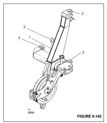
The serial number (1), (Figure 5-142) is on a plate on the right side on the auxiliary single-sheave boom nose.
