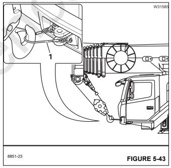
**NOTE:** If the anti-two block switch is deactivated while you tighten the hoist rope, you can override the lockout of the anti-two block switch.
