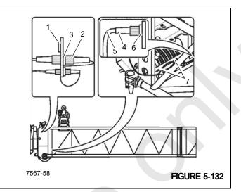
**Connecting the Folding Extension Electrical Circuit**
