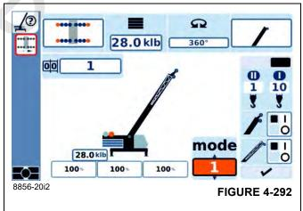
Note that when the RCL configuration screen is used (such as shown in Figures 4-291 and 4-292), the telescoping function is paused (unable to extend, retract, lock or unlock the boom). Once the check-mark is used, the telescoping function resumes.
