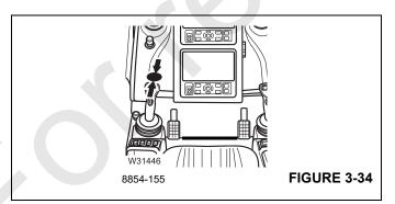
The right control lever will be used for boom lift/lower and luffing boom extension raise and lower.
