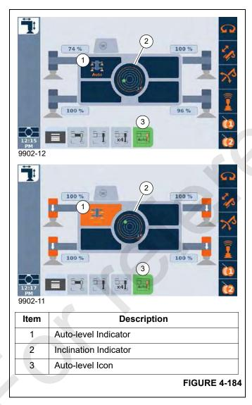
4. To begin the Auto-level function, position the Outrigger Extend/Retract Switch (1), (Figure 3-29) on the left armrest to the extend or retract position, then press and hold the button (1), (Figure 4-185) at the Jog Dial or Navigation Control Pad that corresponds to the Auto-level Button on the screen.
