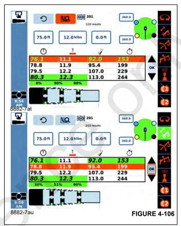
Again referring to Figure 4-106, the second row could be highlighted using the up and down arrows at the right side of the screen. This would be pinning combination 50-51-90 (as seen in the values below the table of values and the graphic of the boom sections). Once a selection is made, the OK button can be used (if the telescoping function has been enabled) to proceed to use the boom configuration in the Semi-auto mode. Another option is to change the rigging information as explained next.
