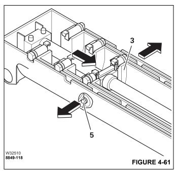
3. Unlocking the telescopic section.
