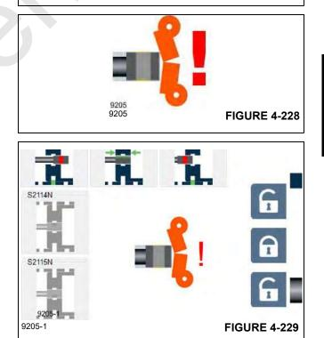
In this triggered condition, the telescoping cylinder is no longer expected to be able to extend. If the extended emergency telescoping mode\_is being used, then it is still possible to still extend the cylinder (such as when the switch is malfunctioning or disconnected), but this should only be
