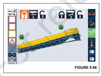
**a.** Use the ODM control pad arrow buttons or jog dial to highlight the unlock icon.
