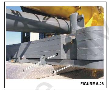
On the counterweight platform, there are four retaining brackets (1), (Figure 5-28), which brings the 3,000 lb tray plate (3), (Figure 5-28) into proper position for rigging and for secure driving.
