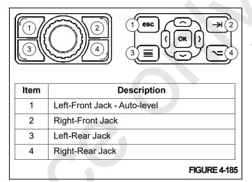
With the two buttons pressed, the Auto-level system will adjust the height of the jacks automatically as it levels the crane. Several adjustments may be necessary.
