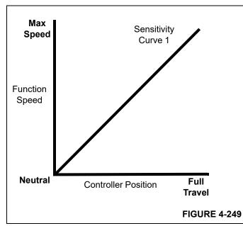
Selecting a sensitivity curve of 2 through 5 (Figure 4-251) causes the function speed to be reduced, from the default sensitivity curve 1, relative to the same controller position over the full travel of the controller (Figure 4-250).
