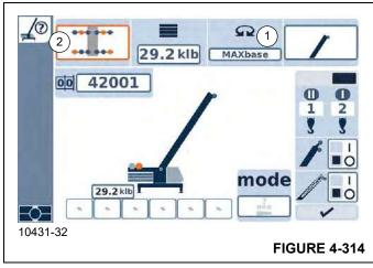
For MAXbase operations the operator can either use the Direct Rigging Code Entry method and enter a MAXbase Load Chart Rigging Code into the Rigging Code selection field (1), (Figure 4-313) or use the Setup Wizard and select MAXbase in the Swing Range selection field (1), (Figure 4-314).
