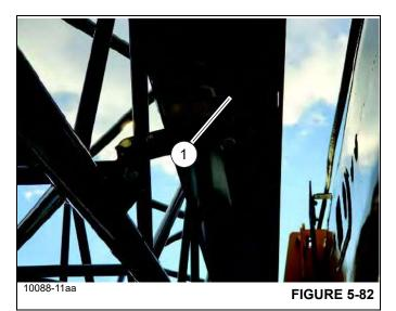
**9.** Make sure the attachment pin (1), (Figure 5-83) and retaining clip are in place that connects the ends of the fly section and the boom extension base section together.
