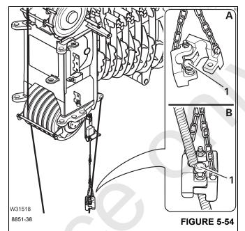
**NOTE:** If you place the anti-two block switch weight around the last rope line leading upwards, less rope will run through the anti-two block switch weight, especially if there is a high number of reevings per lifting operation. This rope line will even be at a standstill if the number of rope lines is even.
