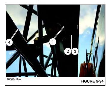
**2.** Make sure the attachment pin (1), (Figure 5-95) and retaining clip are in place that connects the ends of the
