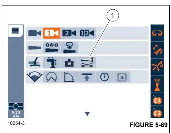
Press the OK button on the ODM navigation pad or press down on the jog dial to select the Boom Extension Deployment/Stowage icon.
