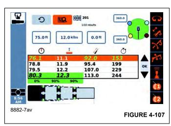
Finally, if it is desired to keep lifts within a criterion such as 75% of the maximum values for the load chart data, then the search can be based on a modified hook load. The modified hook load value would be the hook load divided by the decimal value for the desired limitation such as the following:
