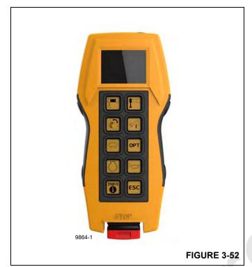
The Remote Control Unit (Figure 3-52) is a rechargeable, hand-held device.
