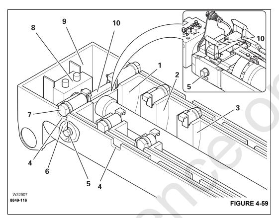
Each telescopic section is equipped with two-section locking pins (7) which are extended by spring force. Refer to (Figure 4-59).
