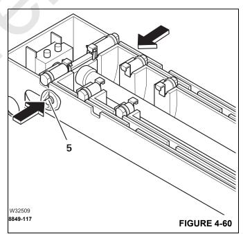
2. Moving and locking the telescoping cylinder.
