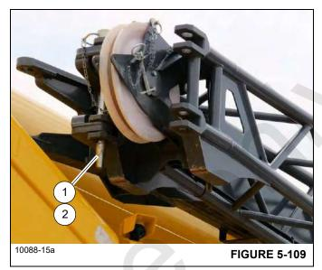
Attach the fly section to the boom extension base section using the connecting link (1), (Figure 5-110). Secure connecting link with pin (3) and retaining clip (2).
