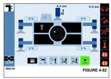
2. Retract the center front stabilizer until the jack is fully retracted.
