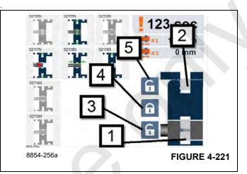
(Figure 4-221) has further explanation for the Telescoping Emergency Program screen. Item 1 is the graphical representation of the tele cylinder pins that connect to a telescoping boom section. When these cylinder pins are considered retracted, an unlock symbol will appear in this location.
