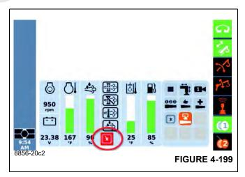
Figure 4-199 shows the symbol (in the red oval) for the Virtual Wall Limitation at the limit. There are similar symbols for the other limitations. Refer to Table 4-9– *WRL Limitation Screen Symbols*, page 4-151.
