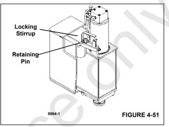
**NOTE:** It may be necessary to jog the outrigger extension/ retraction switch slightly to ensure proper pin engagement.
