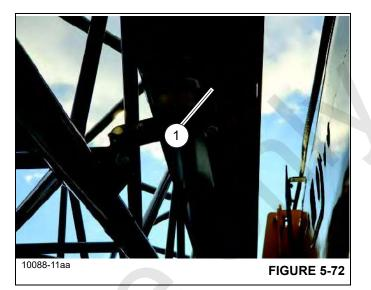
6. Make sure the attachment pin (1), (Figure 5-73) and retaining clip are in place that connects the ends of the fly section and the boom extension base section together.
