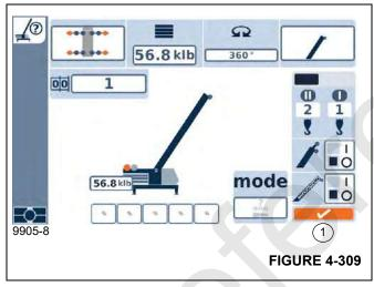
The Monitoring menu is opened and the rigging code is applied.
