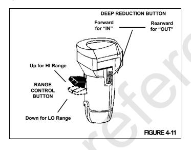
All shifts are made with one lever and a Range Control Button (Figure 4-11) which is used only once during an upshift sequence, and only once during a downshift sequence. Always preselect the range shift. After preselection, the transmission will automatically make the synchronizer range shift as the shift lever passes through neutral.
