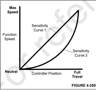
Sensitivity curve 1 (default) is the most sensitive and sensitivity curve 5 is the least sensitive (Figure 4-251).
