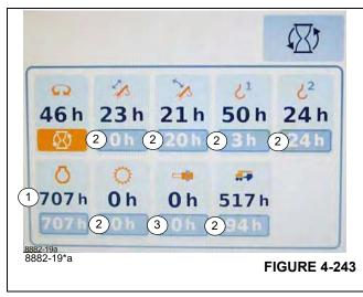
To reset an individual hour meter, use the jog dial to select the time to reset. The selected function will show the icon orange.
