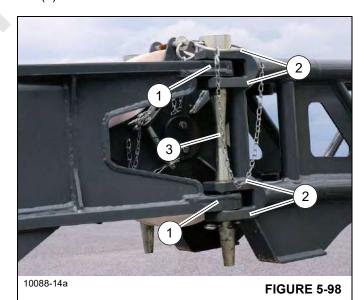
Remove the pin (3), (Figure 5-98) from its holder on the boom extension and insert it into the left side fittings (1, 2). Secure the pin with the retaining clip.
