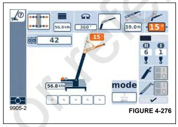
From the RCL Setup Screen, the operator can program the RCL either by entering a rigging code number from the *Load Chart Manual* or by entering the crane configuration using the setup wizard.
