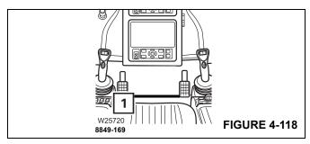
At the initial position, the swing movement will be stopped. At the same time the swing gear hydraulic brake will be applied.
