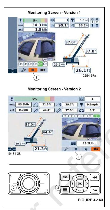
From the Menu Screen, select and confirm the Hoist Camera Icon (1), (Figure 4-164) to open the full screen view of the hoist camera (2).
