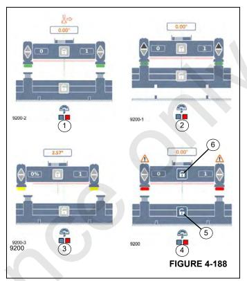
The cylinders are only considered unlocked (able to be raised/lowered freely) at +4.0 or -4.0 degrees. When lowered at that position the crane is then swung to 0.0 degrees where they are raised to lift the counterweight. To unload the counterweight the reverse happens: crane is swung to 0.0 degrees, cylinders extend to lower counterweight onto the deck, crane swings with cylinders extended to +4.0 or -4.0 degrees, cylinders raise without counterweight.
