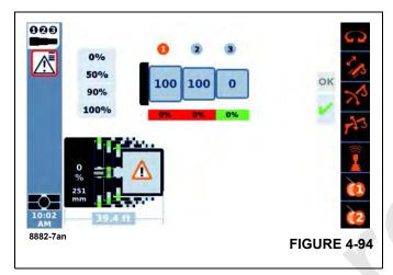
Typically shut-down condition indicates a failure in the components of the control system (such as sensors or modules or communications). If the only indication of faults is for the telescoping function, then the following steps can be used:
