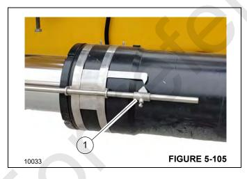
6. In the ODM, verify that the front (Pin #2) and rear (Pin #1) boom extension pins are securely installed. Visually confirm that the pins are installed.
