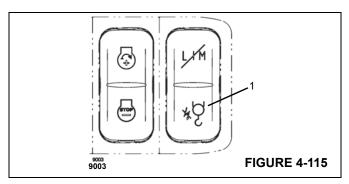
The anti two-block does not bypass the swing brake. It does bypass the swing lockout where swing is not permitted because of:
