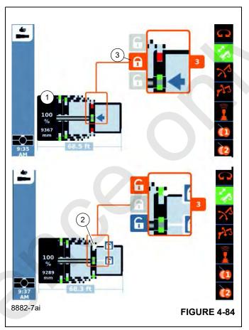
Locking the Telescopic Section for On-Road Driving
