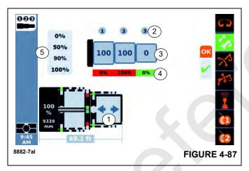
The arrows (1), (Figure 4-87), at some point in the telescoping process, will blink. The blinking is an indication that an unlocking or locking event will occur if the operator holds the joystick in the direction of that arrow for at least 1 second. If this event begins, then the screen will change to the dots (as described for (Figure 4-86)) so that the operator knows that an automated motion or action is again occurring.
