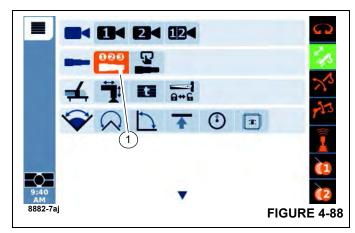
• Verify that the telescoping function is enabled. This is confirmed by the green background for the icon for the telescoping function in the right margin area of the operating display. Refer to (Figure 4-89).
