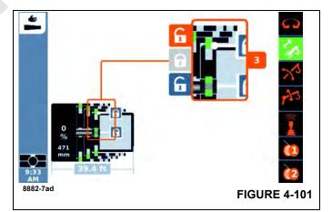
In the Semi-Auto Mode, the unlocking of the telescoping cylinder and boom sections is entirely automated. And when locking is completed in the Semi-auto Mode, the joystick (or other control device) does not affect the position of the telescoping cylinder (the joystick is used to confirm the next command when there is a blinking arrow). In the Manual Mode, the command buttons indicate the unlocking and locking, and the joystick can
