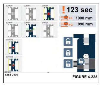
The telescoping boom section is locked (the unlock symbol is not shown near the graphical representation of the section pins - refer to Item 2 in (Figure 4-221).
