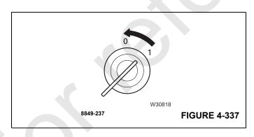
Make sure that no unauthorized persons can operate the truck crane. Refer to *To Secure the Truck Crane Against Unauthorized Use*, page 4-225.
