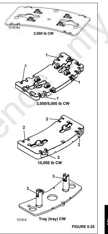
Lift the 2,000 lb, 3,000 lb and 5,000 lb counterweight sections using the four casted sling points (1), (Figure 5-25). These three counterweight plates can be lifted onto the
