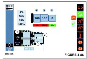
The example in (Figure 4-86) shows the value of 9339 mm for the extension of the telescoping cylinder within the boom.
