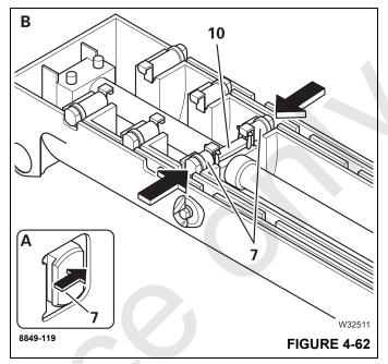
**4.** Telescoping, locking, and setting down a telescopic section.
