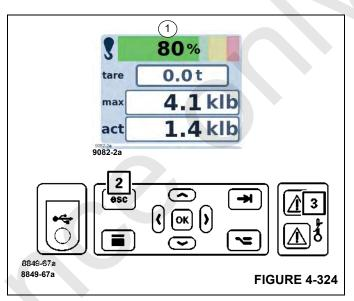
**NOTE:** If the capacity continues to increase, the RCL will reach an overload state and a RCL shutdown will occur.
