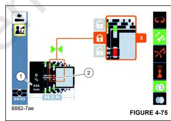
Near a locking point, the symbols (3), (Figure 4-76) show: The direction of travel to the locking point (Figure 4-76):
