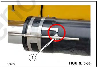
**7.** In the ODM, verify that the front and rear mounting pins are securely installed (Figure 5-81). Visually confirm that the pins are installed.
