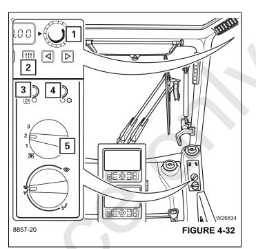
Set the air distribution and ventilation nozzles.
