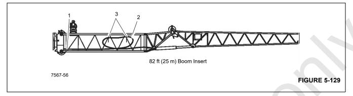
The electric cable (1), (Figure 5-129) is installed in the 26 ft (8 m) insert (2), (Figure 5-129) with the long end of the cable wound on the stowage lugs (3), (Figure 5-129).
