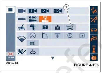
The Boom Extension Deployment/Stowage function screen is used to extend and retract the front and rear boom
