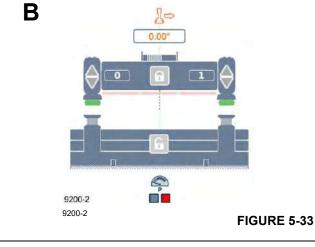
If necessary, correct the displayed rigging mode as follows:
