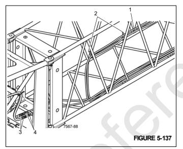
**4.** Secure the hoses (1), (Figure 5-137) to the holders (2), (Figure 5-137) to make sure that the hoses are not damaged during operation.
