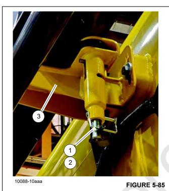
**13.** In the ODM (Figure 5-86), highlight the unlock icon and retract the rear boom extension pin (Pin #1) as follows:
